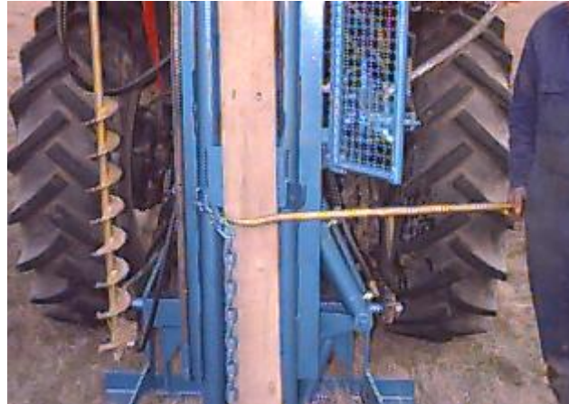
Figure 7 - Driving a Post
